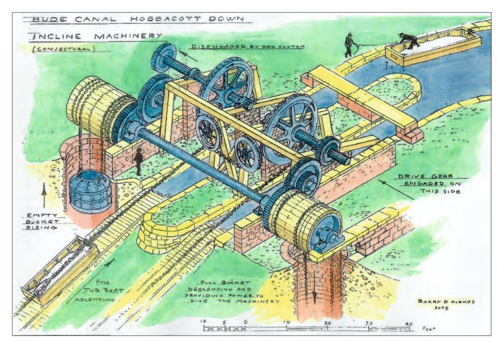
plane and dropped down the well, this being the source of power for the continuous chain. This system was a development of the work done previously by Robert Fulton, Edmund Leach and Earl Stanhope.
